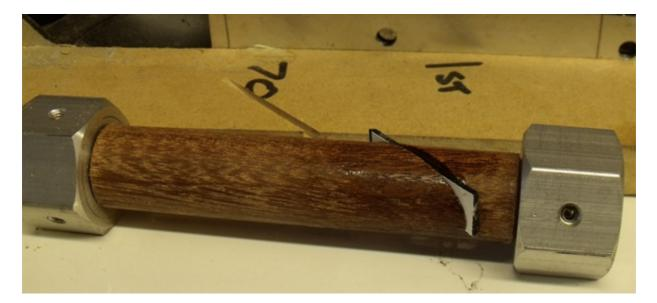
Above is the first cut with an insert already glued in. You will need to make sure that the insert isn't wider than the nuts or the flats of the nuts won't sit flat on the cutting tool table.
