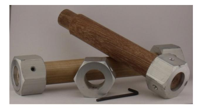
In the above example, two blanks were rounded between centres and then the ends turned down so they fitted in the holes.
