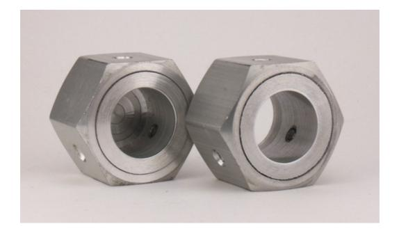
The nuts are simply hexagons with a hole through the middle. One of them in the picture is closed on one side but I have since bored the hole all the way through. On three sides, I drilled and tapped a hole to take small grubscrews. The hole diameter is not critical, but it is easier to use if the hole is similar to a rounded blank. I made mine 20mm Dia.
