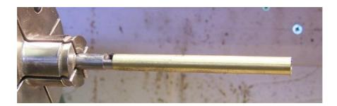
Here you can see why I didn't cut the threads off. I tapped an aluminium tube with the same thread ( 8mm ) and made a handle for buffing As you can see, I am putting loooooooong knurls on everything ( Thanks Joe )
