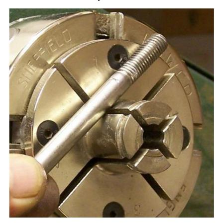
Put the bolt in the chuck and bring up the tailstock. Note that I'm not trying to clamp on the threads. Select a length approx 3/4 the length of the tube and make a mark on the bolt.
