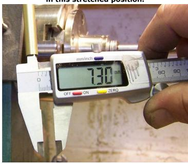
Now the fun part!!! Hold a good clean file in the LEFT HANDED method and with the lathe on quite slow, go for it. Stroke the file left to right in smooth circles. It goes pretty quick so keep checking with the calliper. Use a sharpie to mark any high areas. As the file does not leave the surface, you don't have to worry at all about the washers. Use chalk on the file to prevent clogging and rip out. ( I can't touch chalk,
