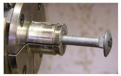
Mount the bolt in the lathe
