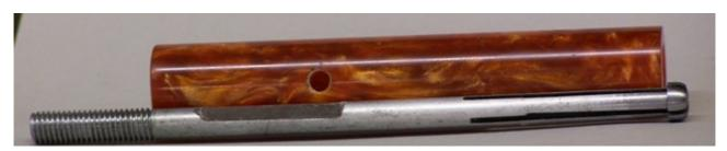
Here is the handle cut to length. Note the tapped hole in the side. This is just for the knob to stop the bolt from rotating while you extract the coupler. Also note that the flat is long enough for the bolt to travel the required distance at least
