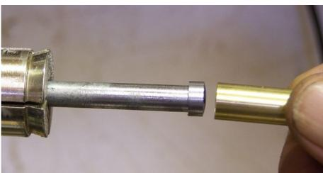
Now file down the bolt head so that the tube just slips over
