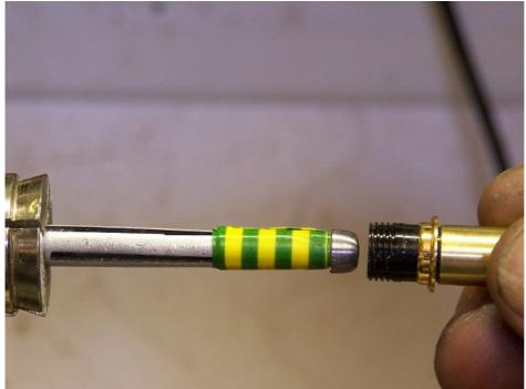
With a little tape, squeeze all the tips together. Now round over the tip and file the diameter down till it fits through the coupler smoothly
